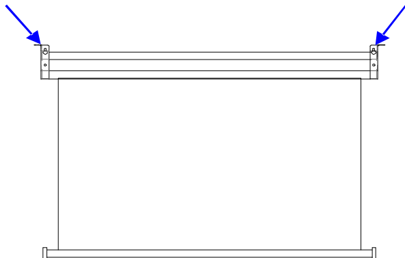
Optional installation method using a chain to hang the screen from the ceiling
