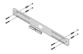
6. Place the bracket on the wall and loosely tighten the screws to secure the bracket. Check with a level and then tighten the screws.
