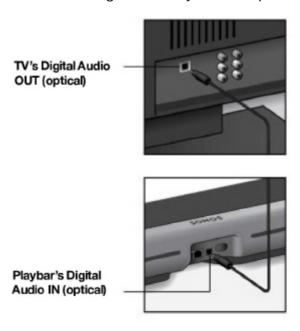
IMPORTANT: Remove the protective caps from each end of the optical audio cable before inserting.
