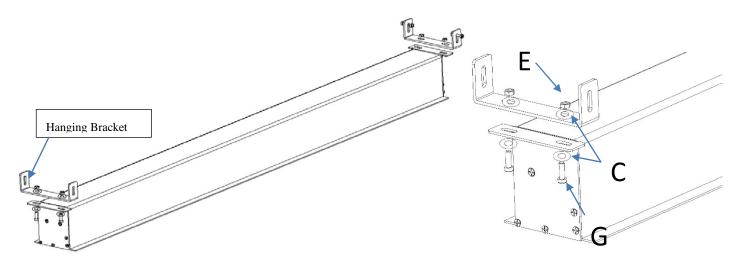
Place the Suspension Bar (B) over the Hanging Bracket (A) and align with the hole as shown below according to the height requirement for your installation area. Secure the Suspension Bar (B) with the M6x20mmScrew (B), M6x13mmx2mmWasher (E) and the M6 Nut (F). Repeat the process for the other side.
