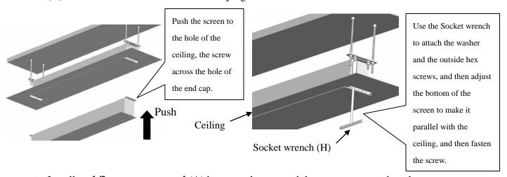
6. Install **end flange cover panel** (A) between the gap and the screen to complete the installation.
