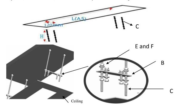
5. Push the screen up into the space. Use the **threaded rods** (C) to attach the screen assembly to the ceiling. The **hexagonal screws** (E) will connect the screen to the rest of the assembly. Once firmly in place; use the **nuts** (F) to ensure a firm connection. Use the **socket wrench** (D) to make sure that the bolts are firmly tightened.
