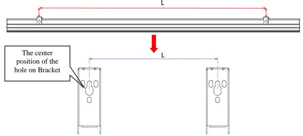
2. Drill the holes and insert the **Anchors** (**E**), and fixed the bracket into the wall with **M5.5 screws**(**D**), then loosen the screw under the **Bracket** (**A**) counterclockwise.
