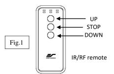
3. RF Remote Control (Item B): The radio waves eliminate the need for a direct line of sight and has a range of 100 feet.
