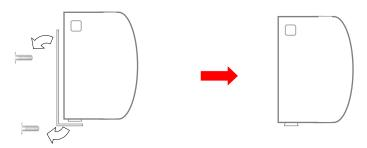
4. Attach the screen to the **Bracket** (A) by inserting the top of the case to **Fix Plate 1** and securing the back of the case to **Fix Plate 2**. Make sure the case slots are securely attached to the **Mounting Bracket** (A)
