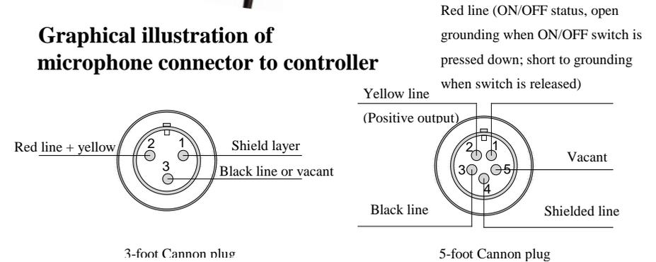
Note: In most cases, Cannon plug is for connection to microphone jack on front panel of the controller; 6.35mm plug is for connection to microphone jack on rear panel.
