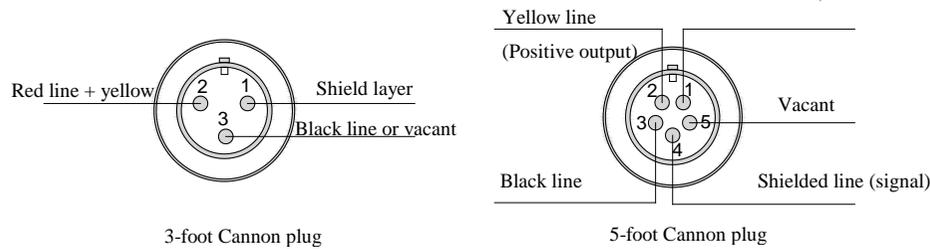
Note: In most cases, Cannon plug is for connection to microphone jack on front panel of the controller; 6.35mm plug is for connection to microphone jack on rear panel.
