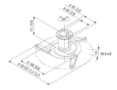
The metal arms are adjustable and fit virtually all projectors equipped with screw connection. Using the handy click in/out system, it is easy to attach or remove the projector, for instance for service purposes. Whether it be for presentations, or for watching movies, this universal projector mount will come in very useful. It avoids the necessity of finding a table or temporary support for the projector.
