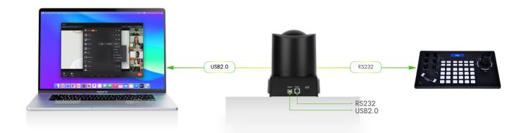
The camera supports RS232 serial port and can be equipped with a remote control keyboard to control the camera functions, such as pan, tilt, and zoom.
